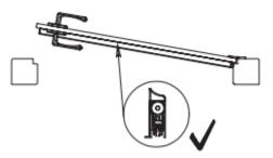
2. If you install the profile on the glass door without frame place activating kit fitting on the glass wall on the closing side of glass door.
